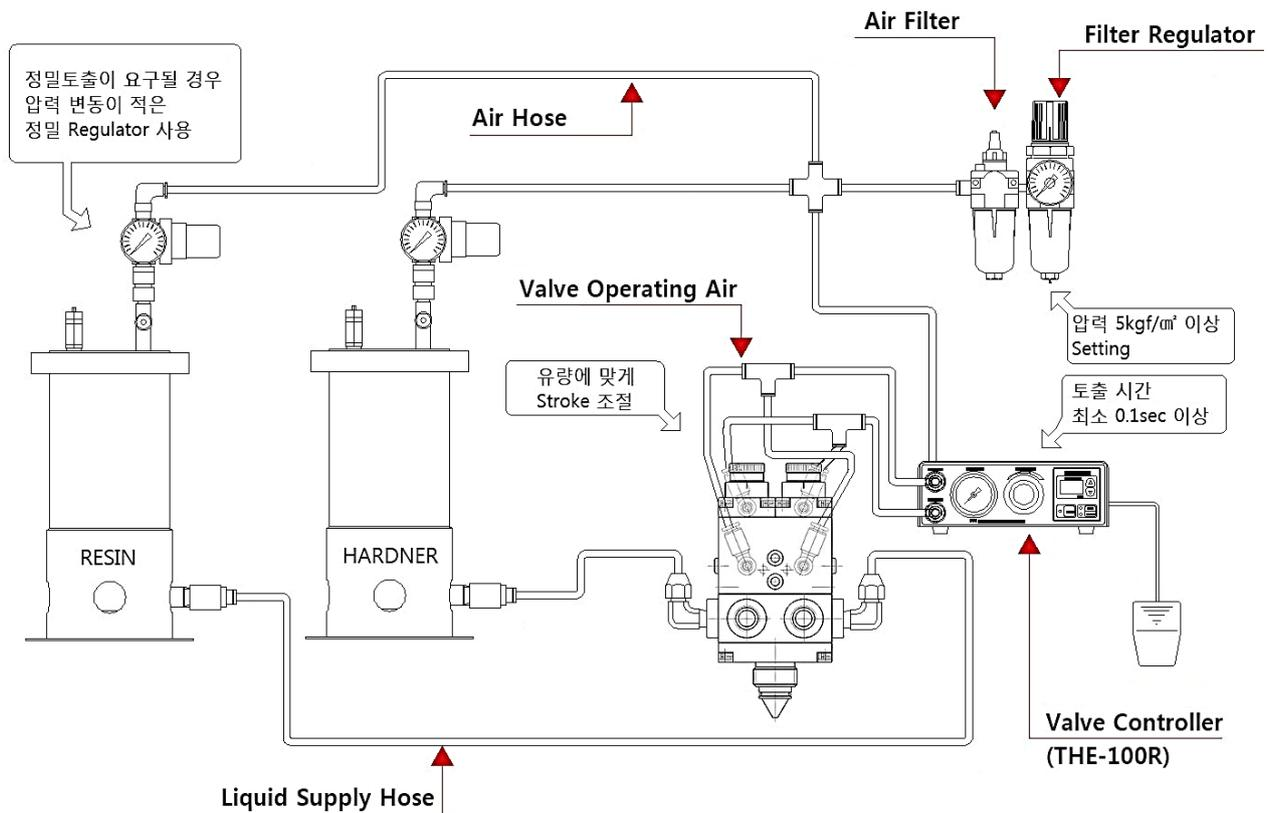
Figure 4. TDV-300T Typical Installation Example
