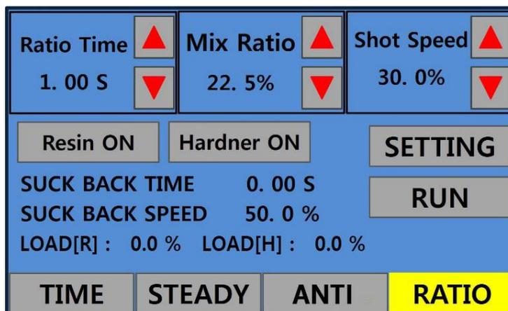
Figure 10. Ratio mode main screen
