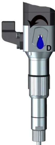
When the pump and the controller's settings are finished, before applying the solution to the product, rotate the D(Vent Knob) as the arrow direction one to two rounds to discharge the bubbles and some liquid(about 5~10 seconds). When it is confirmed that the bubbles are all eliminated, then close it off again.
