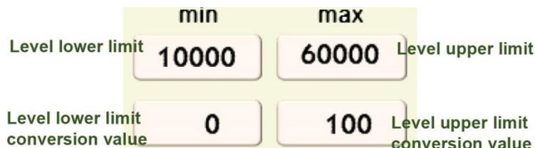
**Level lower limit :** When the water level is the lowest, input the digital value received from the level sensor.
