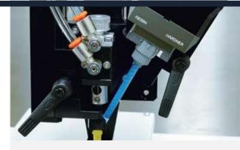
A control device that can be applied to equipment such as desktop robots, articulated robots, inline systems and etc. to select the method of dispensing and to control the dispensing volume.
